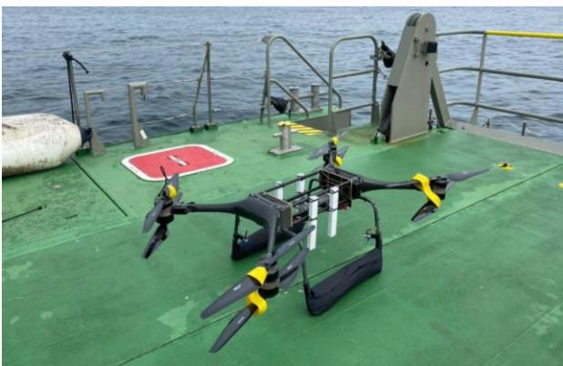
Fig. 2. Heavy-duty Minerva drone used for water exercises.
