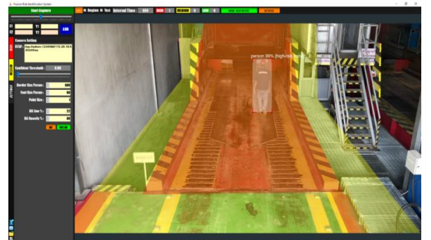
Fig. 5. The truck dumper control system with YOLO as a module for human detection and the developed risk-level identification
