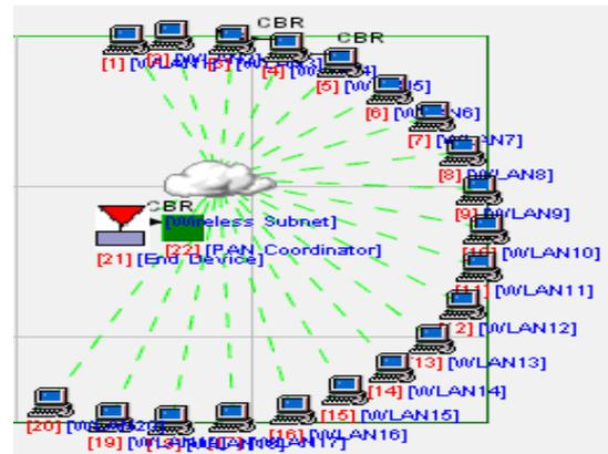
Fig. 12 Circular topology Simulation Model between IEEE 802.15.4 and IEEE 802.11b
