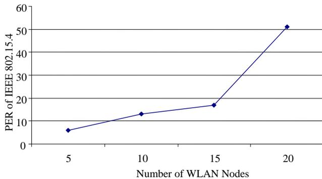
Fig .11 PER of IEEE 802.15.4 for Grid Topology with 20 nodes
