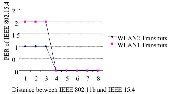
Fig 7. PER of the IEEE 802.15.4 without considering the power spectral density of the IEEE 802.11b
