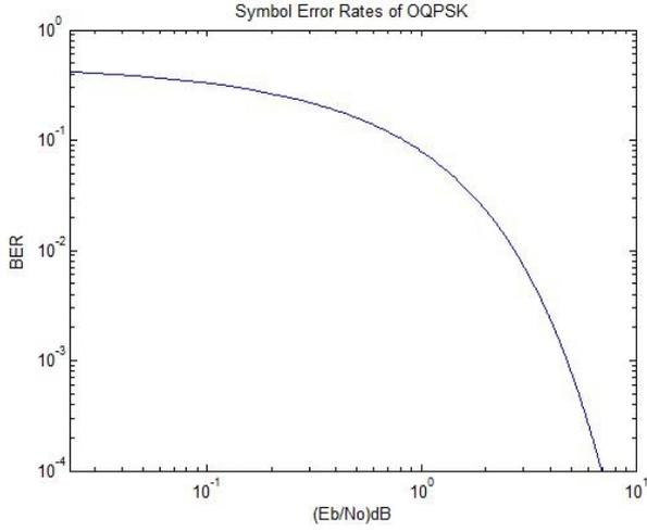
Fig. 3 Theoretic Bit Error Rate of OQPSK
