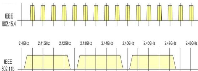
Fig. 1 Channel allocations of IEEE 802.11b and IEEE 802.15.4 technologies
