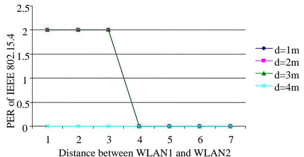
Fig. 9. PER of the IEEE 802.15.4 for various Distances  $d$  between WLAN1 and WLAN2
