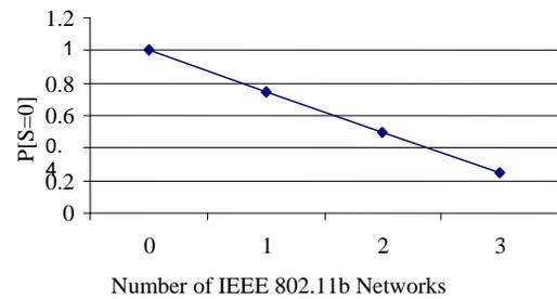
Fig 2. Analytical results of P[S=0] while one IEEE 802.15.4 network coexist with multiple IEEE 802.11b networks
