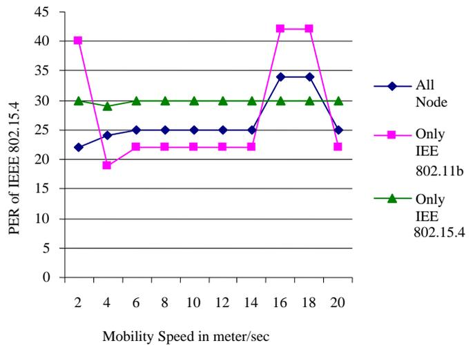
Fig.17 PER of IEEE 802.15.4 with the Mobility model (various speeds) for Grid topology
