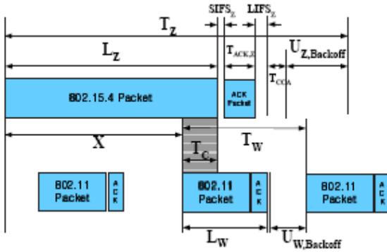
Fig. 4. Interference model between IEEE 802.15.4 and IEEE 802.11b
