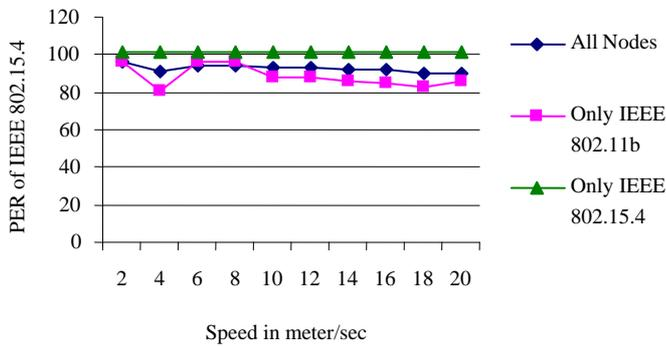
Fig 15 PER of IEEE 802.15.4 with the Mobility model (various speeds) for Circular topology
